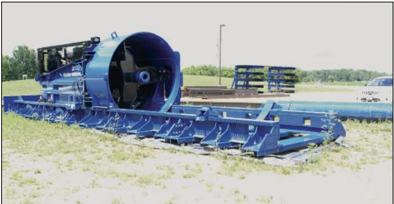
The American Augers 84/96-1800 can bore 96-inch-diameter holes. (Photo courtesy American Augers Inc.)
