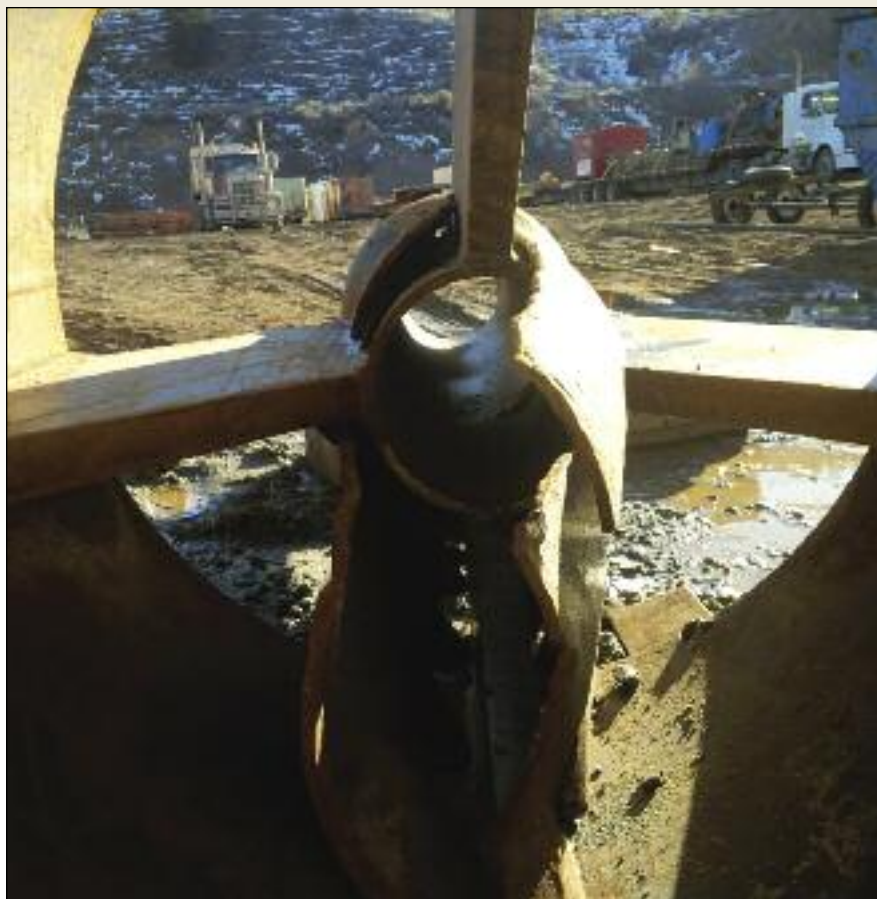
A project in Maple Ridge required a specially designed burst head.
