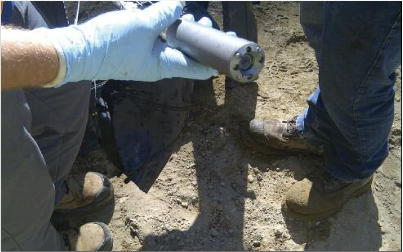
The LDS1000 system, which includes a camera and microphone, was used to inspect a watermain in Whistler.
