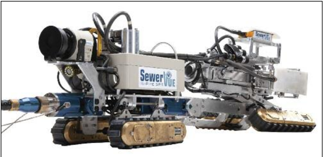
The SewerVUE Surveyor is a multi-sensor robot that utilizes CCTV, LiDAR and PPR.
