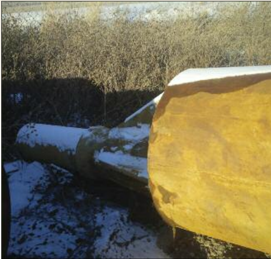
KAB designed an eccentric burst head for the Maple Ridge project.
