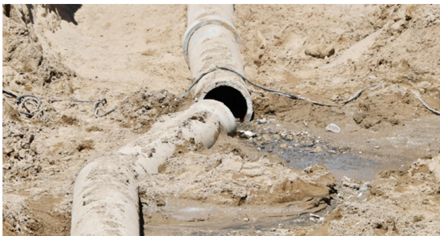
RIDGECREST, Calif. - A formerly straight section of pipe broken by shifting earth during a 7.1 earthquake that shook Southern California in July 2019, cracking buildings, breaking roads and causing power outages. The quake, centered 11 miles from the Ridgecrest area, is the largest quake to hit Southern California in at least 20 years. It was followed by a series of large and small aftershocks, including a handful above magnitude 5.0. (Credit: Gene Blevins/ZUMA Wire/Alamy Live News)
